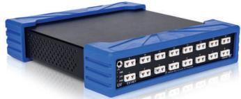
The EX1401 delivers accurate and highly repeatable thermocouple  $(\pm 0.20^{\circ}\text{C})$  and voltage measurements by implementing fully integrated signal conditioning, 24-bit ADC's, and independent Cold Junction Compensation (CJC) on a per-channel basis.
