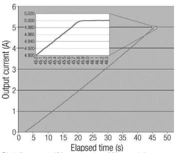
This plot illustrates an actual 5 A current change into an 8.6 H superconducting magnet. A smooth, 95 mA/s ramp is shown with minimal overshoot highlighted in the detail area. (Output current monitor measured at 58.88 Hz rate with a HP 34401 – data multiplied by  $10 \times$  to obtain output current results.)
