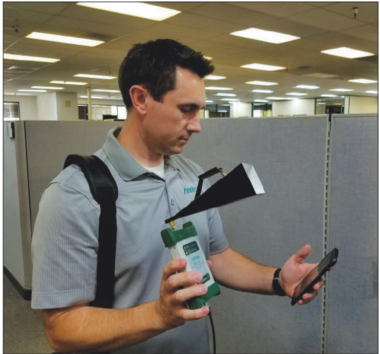
Figure 4. Millimeter-wave indoor coverage mapping solution.
