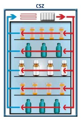
These chambers are used to test and store a wide range of products in specific temperature and/ or humidity conditions.
