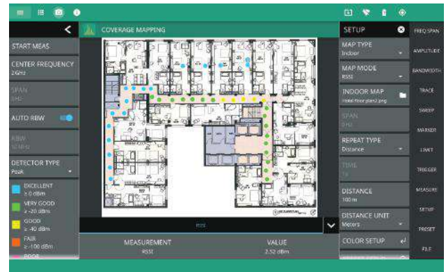
Typical Result Screen for Indoor Coverage Mapping
