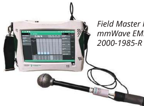
EMF Results Show Power from each Antenna Axis and Summary Results for Peak and Average Power over a Defined Time Period
