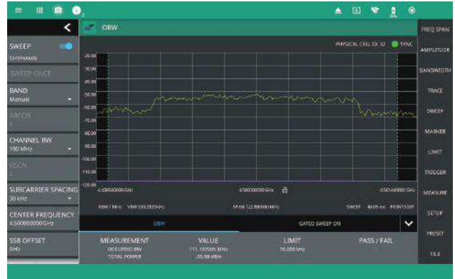
Automated Occupied Bandwidth Measurement Result for a 100 MHz 5G NR Radio
