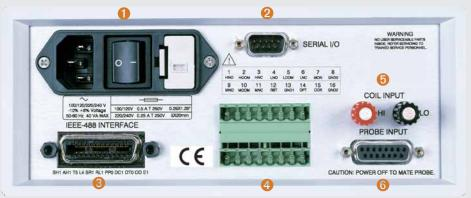
The Model 480 terminal block has connections for external reset. With this feature. a foot pedal or programmable logic controller (PLC) can be used to start a new measurement cycle. The external reset is TTL-compatible and a logic low will activate a reset. The signal is internally pulled up to allow operation with a simple switch closure between pins 12 and 13.
