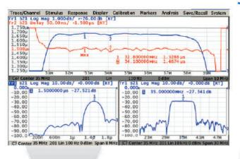
Time domain analysis allows measurements of SAW filters such as the time delay and feedthrough signal suppression.
