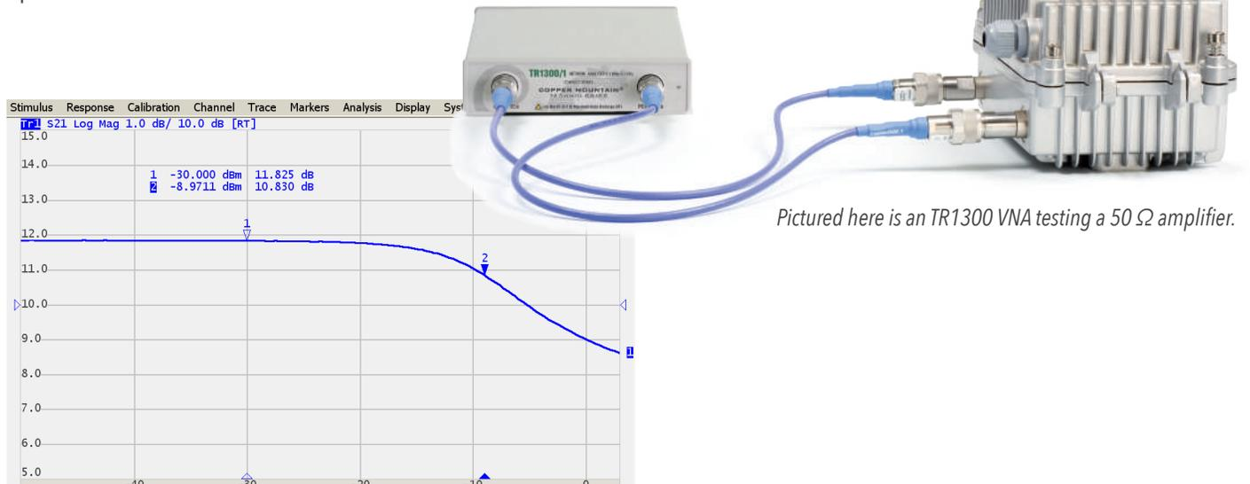
*Pictured here is an TR1300 VNA testing a 50  $\Omega$  amplifier.*
