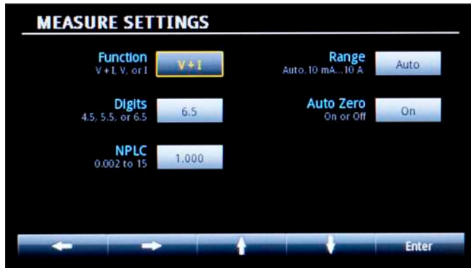
Figure 5. Configure the readback measurements exactly the way you need them using a Measure Sub-screen.
