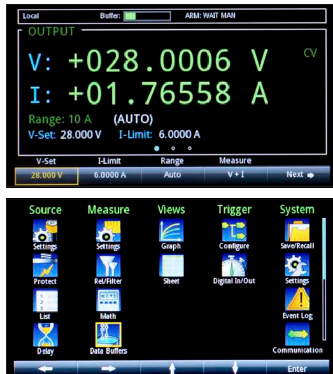
Figure 3. Adjust voltage, current, the current range, the measurement mode, protection levels, and other functions from the home screen.
