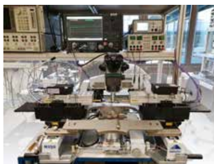
b) Example of system implementation for load-pull measurements using MMW-STUDIO; 2x VMU201802 are mounted directly on WR10 OMLN5260-60003 extender.
