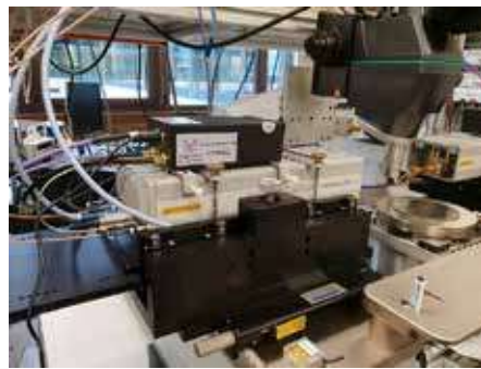
b) Mounting detail of a VMU201802 on an OML N5260-60003 extender.
