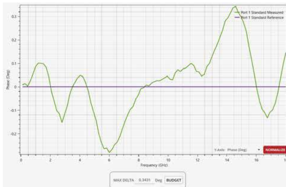
Figure 1. Normalized phase response between user-measured and factory-measured standard
